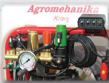
For spraying, the high-pressure piston diaphragm pump is used. The Agromehanika pumps are distinguished by their reliability and a high-quality manufacture, which is confirmed by the 3-year warranty period and flawless
